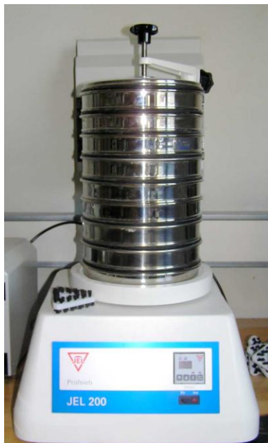
Figure 2.21 Mechanical sieve shaker ( https://commons.wikimedia.org/w/index.php?curid=6360346 )
