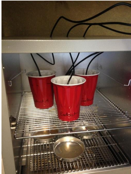
Figure 2.32. Substrate in cups with sensors placed in drying oven to allow for the evaporation of moisture content
