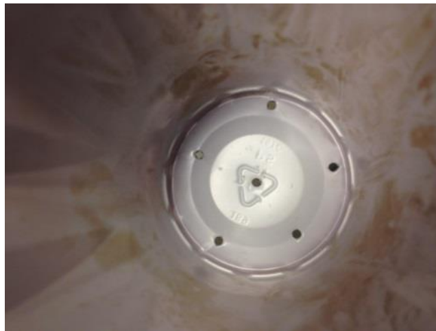
Figure 2.31. 16oz cup with holes used for sensor calibrations
