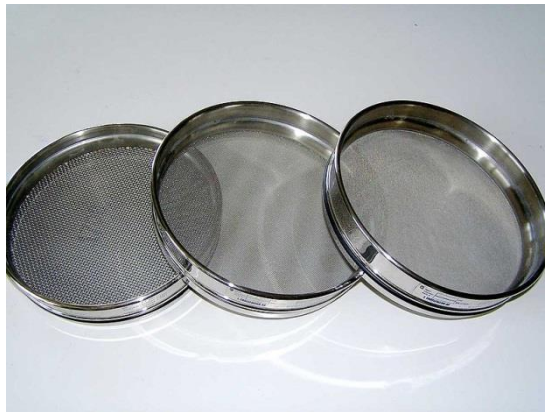
Figure 2.22 Sieves with variable mesh sizes used in the sieve analysis ( https://commons.wikimedia.org/w/index.php?curid=650352 )
