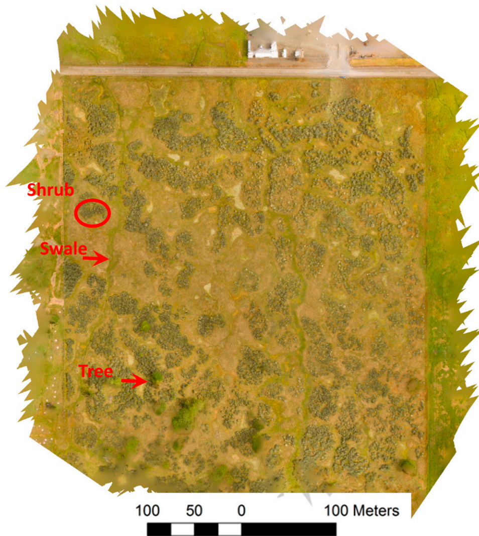
Fig. 4. An orthomosaic of the vernal pool region of the Whetstone Savanna Preserve in southern Oregon generated from aerial images collected using a small drone (DJI Phantom 2 Vision+). To the north is a rural road and light industrial complex. There is a fence line along the west side that is evident as a linear disruption in the vegetation. Along the east side is an agricultural field, and to the south is oak savanna. Examples of shrub, swale (vernal pools), and trees are indicated. Hummocks are regions that generally border between swales and shrubs.
