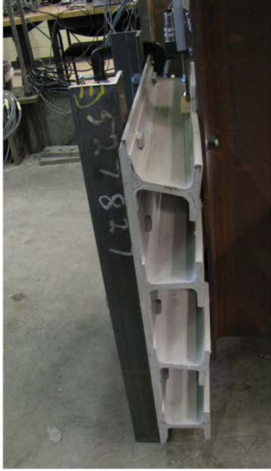
(a) Modified ZellComp deck-to-stringer bolts below web
