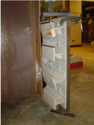
(a) Modified ZellComp deck-to-stringer bolts above web
