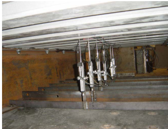
Fig. 8: Deck displacement measurements
