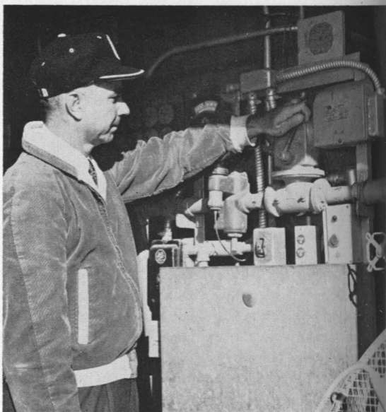
D. L. Calderwood ignites the burner on the experimental rice dryer in studies to determine better procedures for operating commercial rice dryers.
