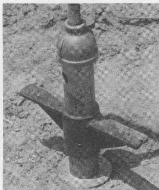
Figure 3. Soil sampler replaced in hole made when 0-to-3-inch soil core was removed before taking a core from the 3-to-6-inch section.
