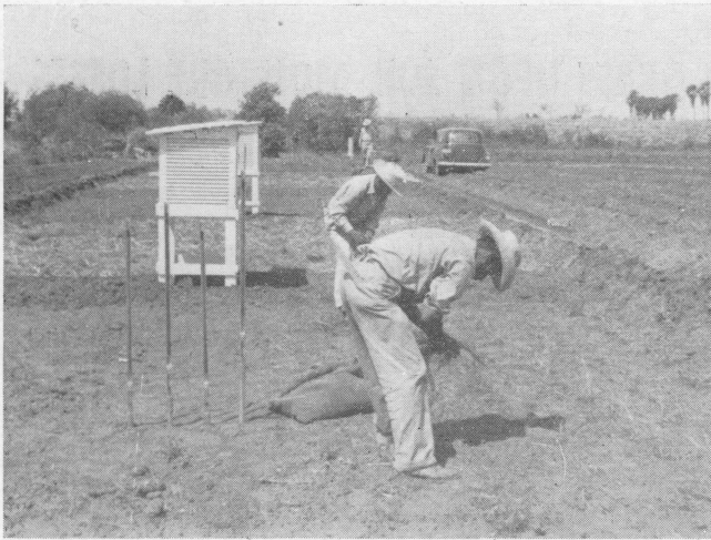
Figure 1. Grass plots being sprig sodded initially with Medio bluestem grass. Tensiometers were set at depths of 9, 18, 30 and 42 inches in each treatment for measuring soil moisture tension changes within the soil profile.
