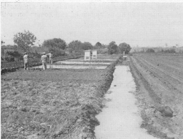
Figure 3. Overall layout of plots, instrument shelters and method of applying irrigation water. All soil-moisture samples were taken within the center area of each plot.
