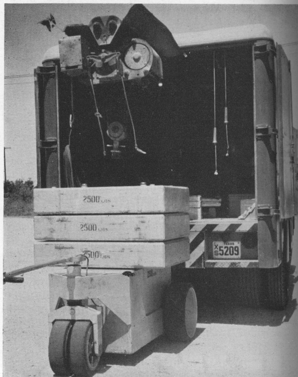
Figure 5. Truck unit and a 2,500-pound dolly loaded with three standard weights of 2,500 pounds.
