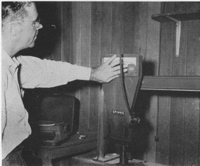
Figure 8. State sealer seals the scale after it has been tested and found to be in tolerance.
