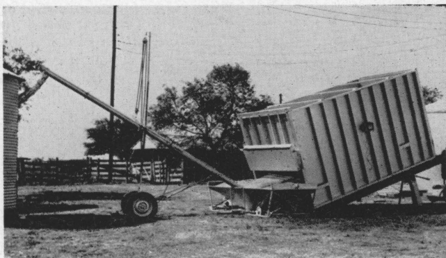
Figure 5. A heavy duty hydraulic wagon dump was one method used to unload the portable batch dryer.
