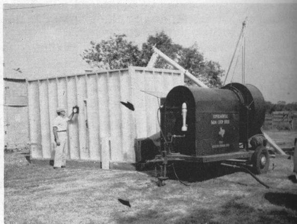
Figure 3. This portable batch dryer, used in the studies, consisted of a drying bin 7 by 14 feet with walls 6 feet high. A perforated steel floor separated the drying bin from an air chamber. Seed were loaded to the desired depth on the drying floor and heated air was forced into the air chamber and through the seed until the moisture content was reduced to a safe limit.
