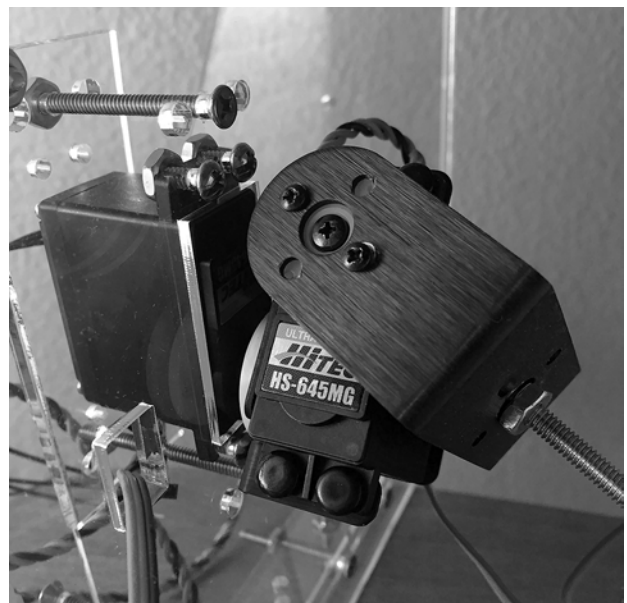
Figure 6. Anodized aluminum brackets for 2 axes rotation attached to two high torque servomotors.
