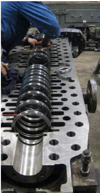
Photo 8 : Pictures shows an 14 stage pump stationary wear ring made of PEEK material inserts (assembly in progress)
