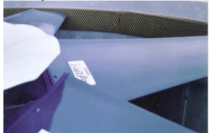
Photo 9: A fin fan blade upgrade with tip seal installation to improve efficiency
