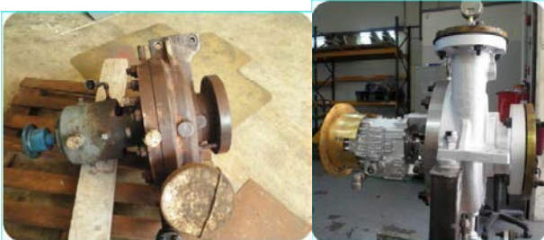
Photo 6: Pictures show a pump before and after upgrade
