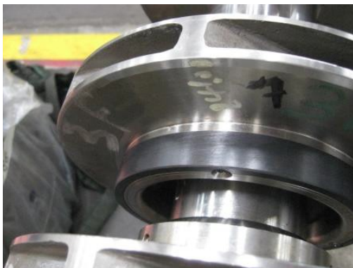
Photo 7 : Pictures show the multistage pump impeller wear ring and stationary wear ring made of PEEK material and insert.
