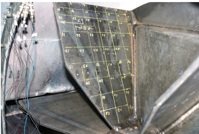
Figure 8. Blade of the shredder fan under testing.
