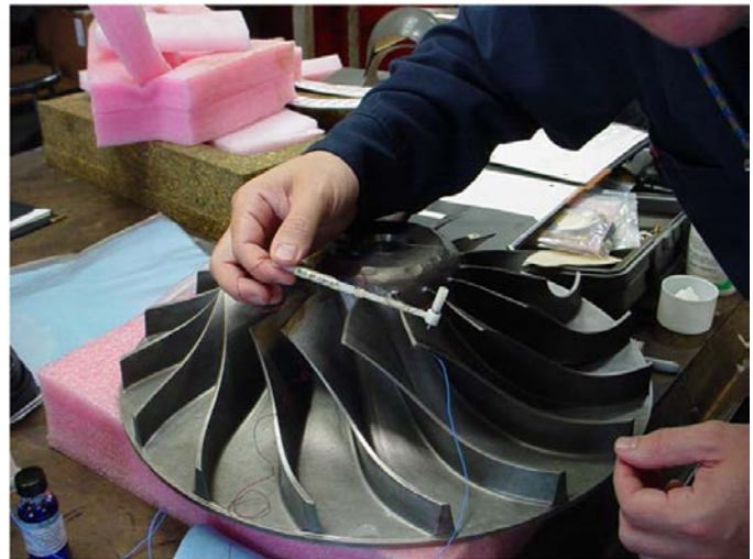
Figure 22. Impact testing of compressor impeller blade
