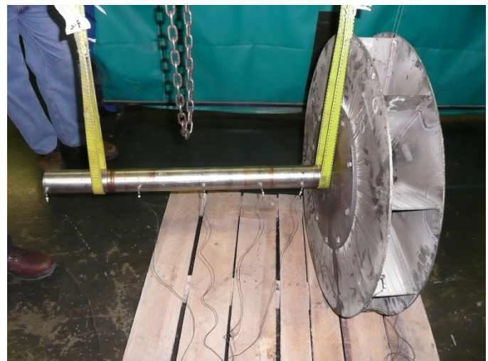
Figure 18. Rotor of small blower horizontally supported for impact testing.
