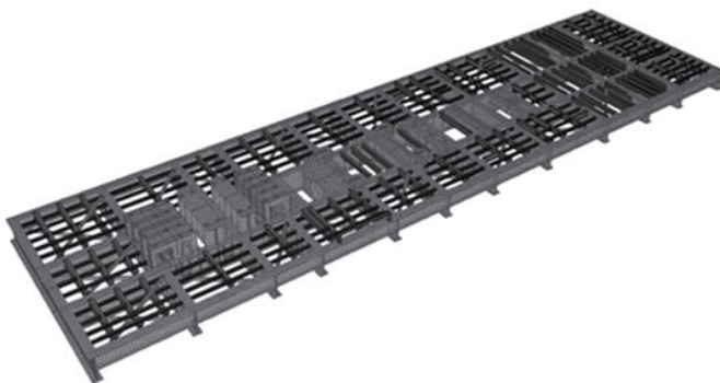
Figure 23: GTG Module – Machinery Deck
