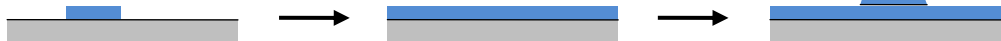
Figure 2-6. Schematic representation of the three general modes of growth. (a) Layer by layer growth occurring when wetting of the substrate is favoured, (b) island growth, and (c) the intermediate Stranski-Krastanov growth mode in which after an initial wetting phase, island growth occurs.
