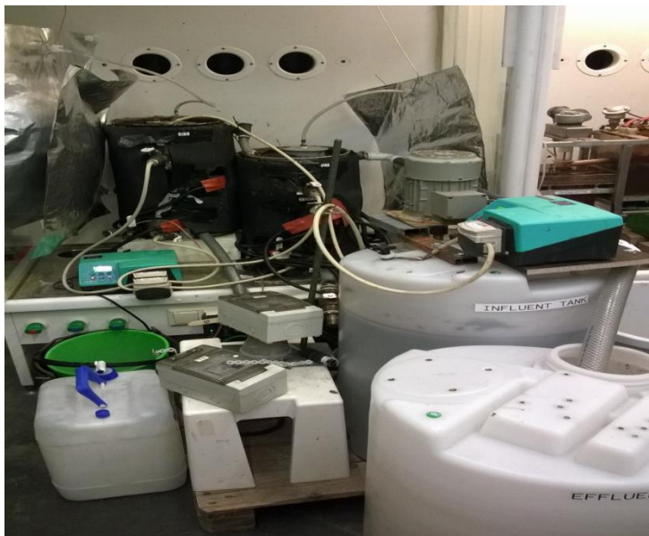
IMAGE 3.3 UASB apparatus in Savonia . From left to right are reactor 1, reactor 2, Effluent. Photograph Antti Koskenlahti, 2017
