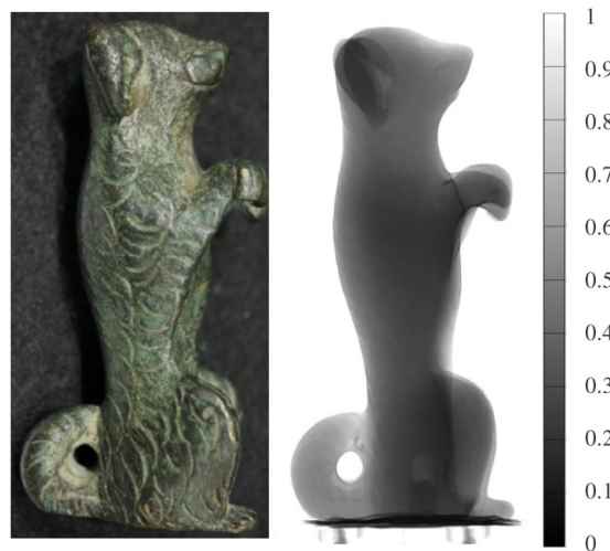
Figure 2.15: Photograph and neutron radiograph of an bronze dog statuette (7.5 cm x 3.5 cm) [22]
