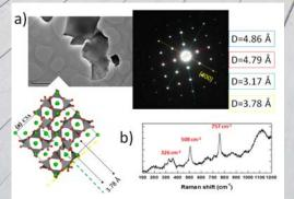
The aluminate content increases with increasing molar ratio A:C. For a 1:3 molar ratio, the highest content of calcium aluminate was obtained for all dross studied. For this ratio, the majority aluminate is C<sub>3</sub>A (tricalcium aluminate) whose content is 85% and 87% for dross Al-1 and Al-3 respectively, and 72% for dross Al-2
