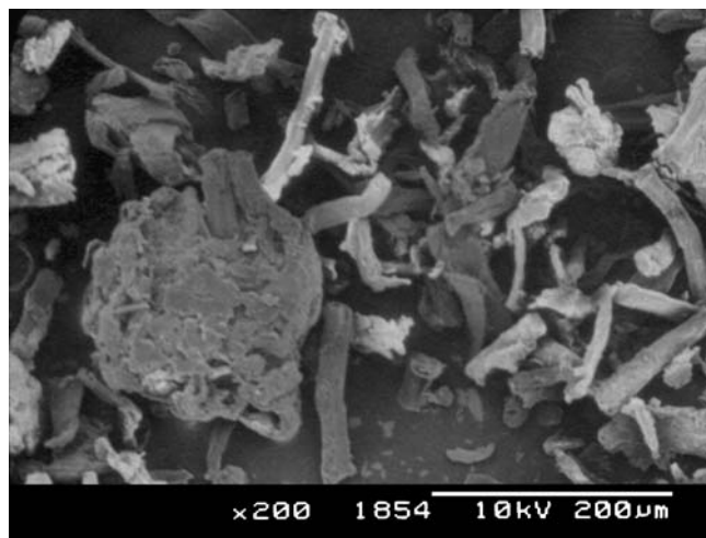
Fig. 2. SEM picture of Vivapur 102
