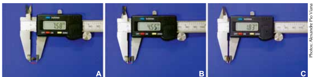
Figure 10. Measurement of sour passion fruit seeds. A – longitudinal diameter; B – transverse diameter; C – thickness.
