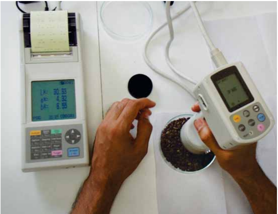
Figure 9. Determination of the color of the seeds using a digital colorimeter.
