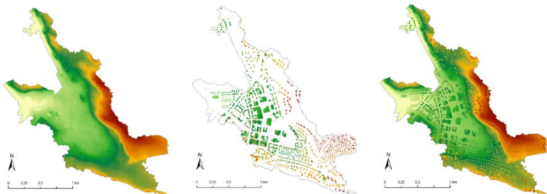
Figure 22. Mosaicking the original terrain DEM (left) with the building DEM (center) resulted in a complete DEM (right).
