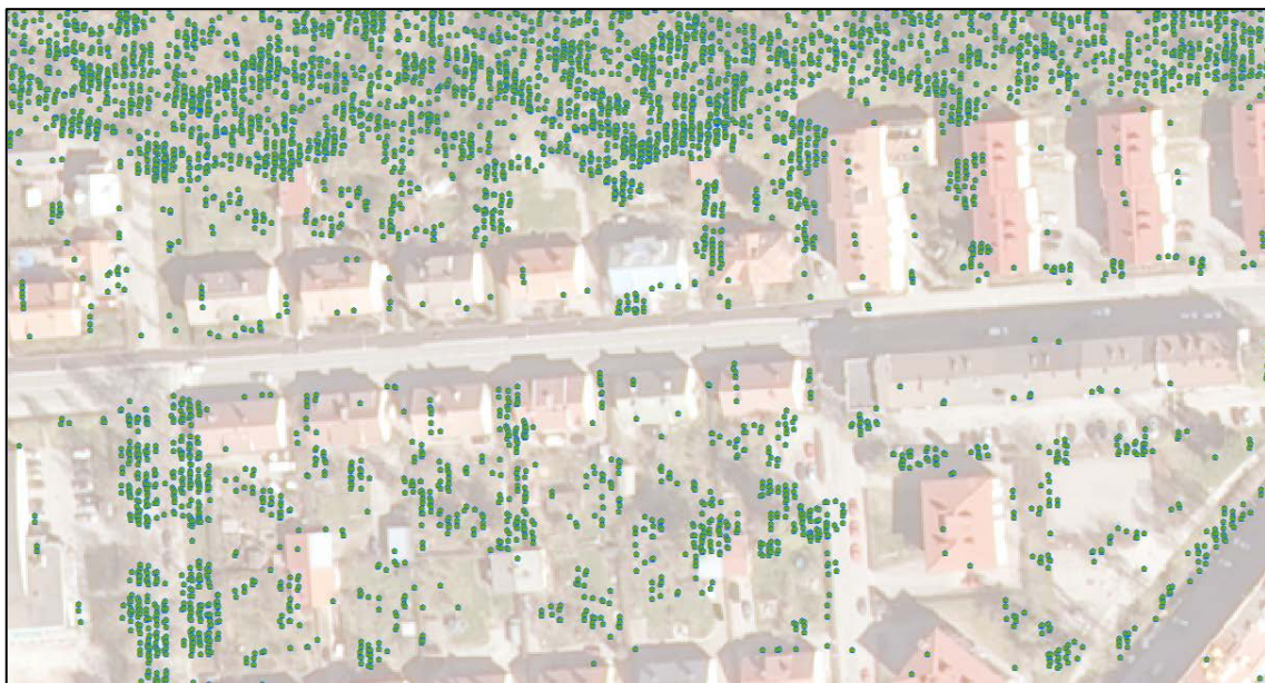
Figure 7. Laser scanning data, with only Class 3 (Low vegetation) points set visible on top of an orthophoto.
