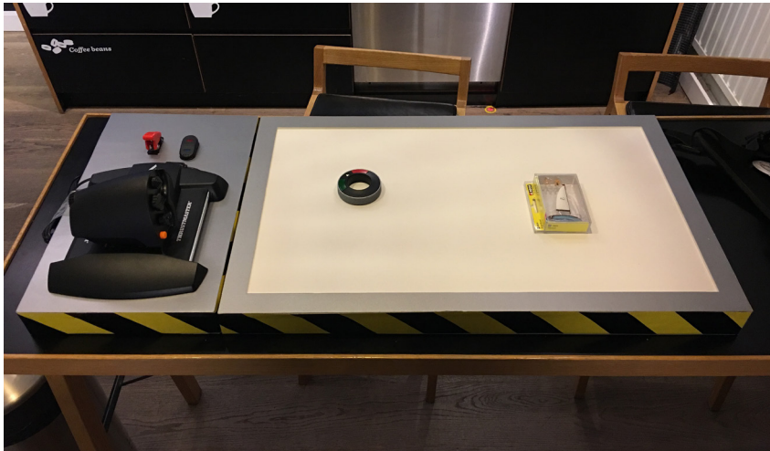
Figure 2. Supervisory Control Interface for Semi-Autonomous Cargo Vessel Prototype (i)
