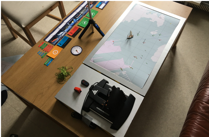
Figure 3. Supervisory Control Interface for Semi-Autonomous Cargo Vessel Prototype (ii)
