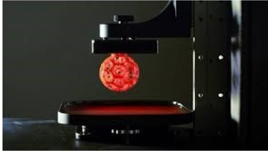
Figure 35. Part that can not be manufactured by conventional processes [32]
