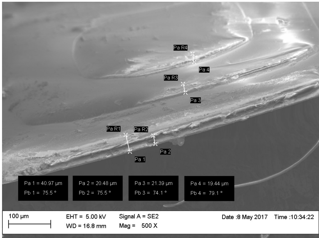
Figure 54. Analysis of the thickness. Four layers of 20 μm each
