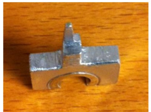
Figure 25. Platform used. Device to which the first layer is attached to
