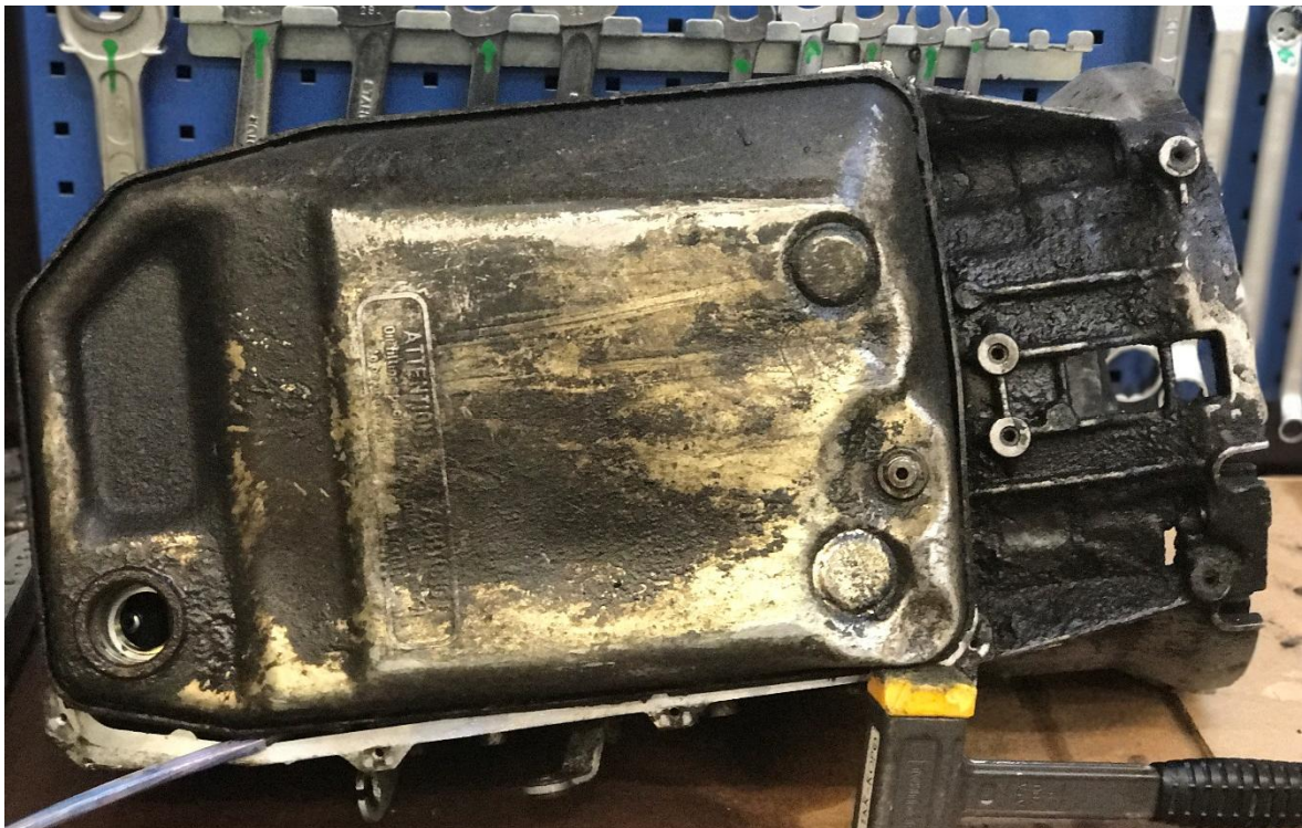
Transmission oil pan - first step for disassembly
