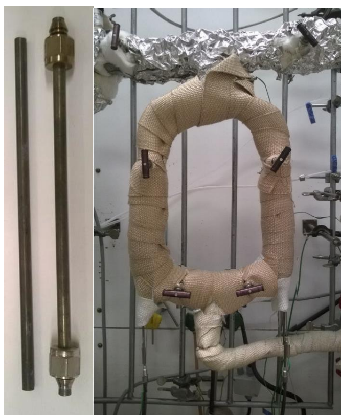
Figure 27: Picture of a) reactors with and without fittings and b) test setup.
