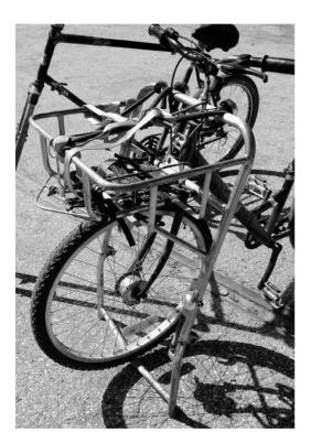
Figure 7: Metal scraps were collected and welded as a protective cover against strong impacts.
