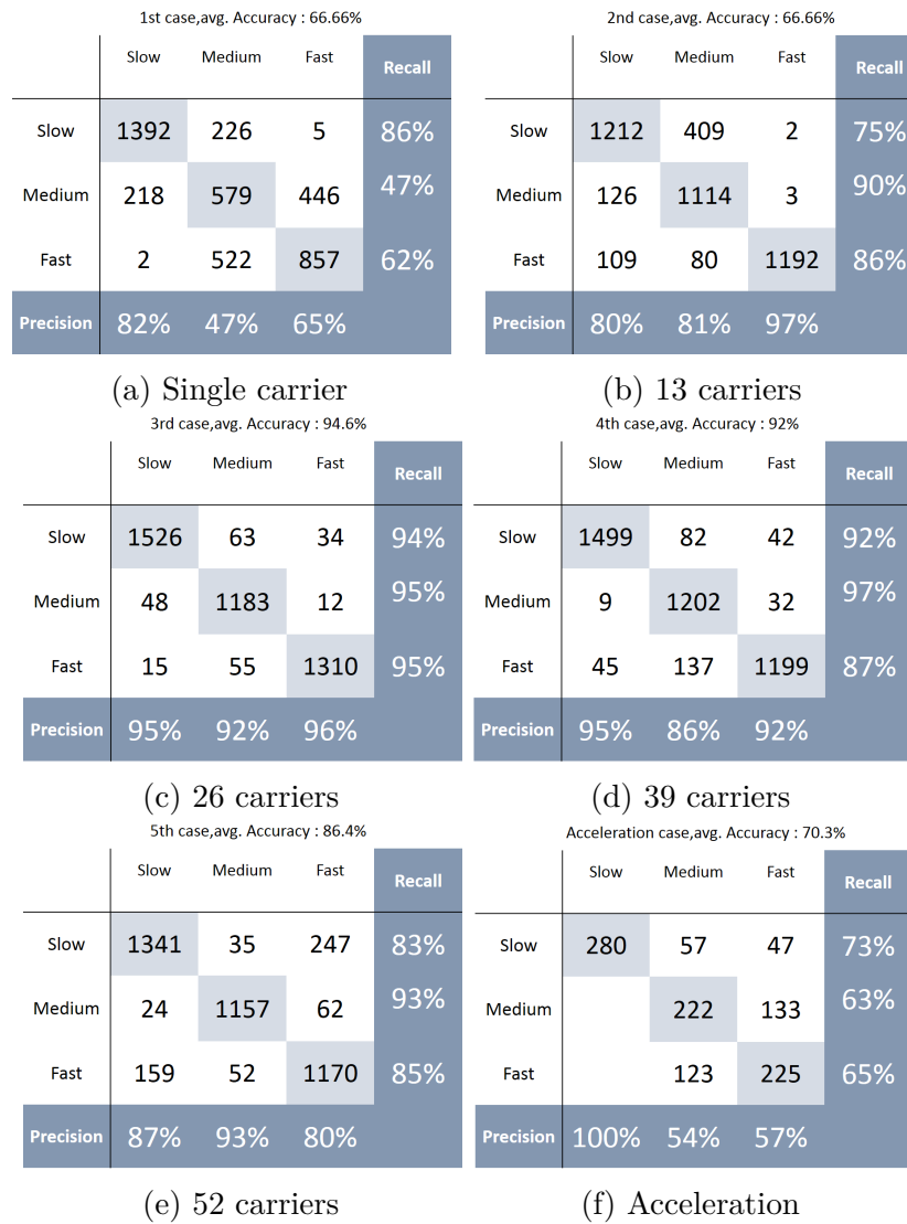
Figure 16: Confusion matrices of three walking speeds recognized by K-NN classifier for all six cases have been indicated in this figure. Average accuracy is also shown for each case.
