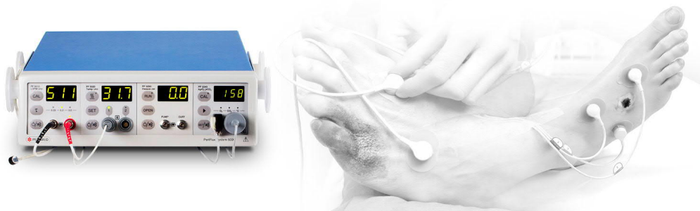
Figure 2.8: PeriFlux System 5000 device (on the left) and example of the skin measurement probes installation (on the right). Reprinted from [10].
