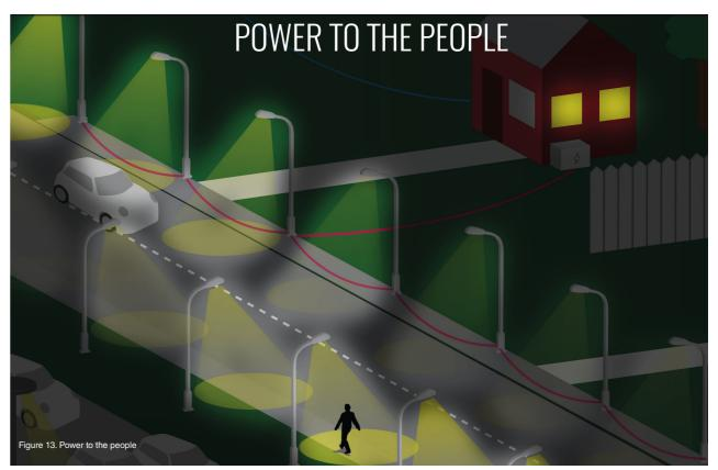
Houses are sharing the electricity with public street lighting. The house has a battery, that can be used to used to light the lamps when electricity is expensive. Citizens have better control of the light properties such as brightness and gain possible savings of electricity themselves.
