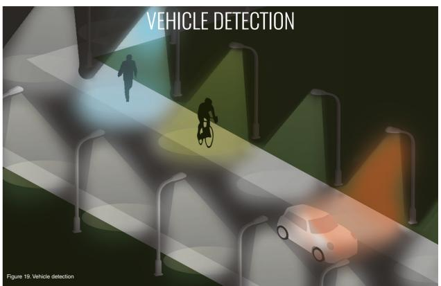
Lights changing color depending on the speed and type of a vehicle. Collisions could be avoided by seeing type of vehicle from a distance.
