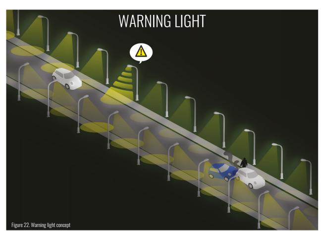
Light is communicating by blinking in case of accident or other distrubance on traffic. Sensors can pick up unusual activity, such as blockage on the road and warn approaching car depending its speed.
