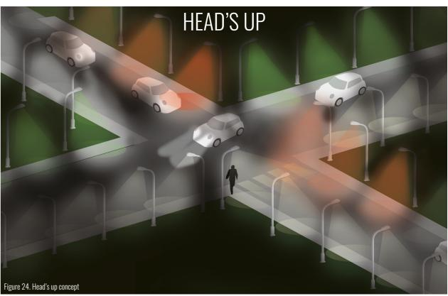
RGBW LEDs are used to guide traffic by communicating to who should go forward and who should not pass. This solution could work as it's own or as an addition to traffic lights.
