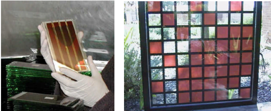
Figure 14. Left picture: Dye-sensitized solar cell tile from the STI production line (Source: http://www.sta.com.au/newimages/hhttp12.jpg ). Right picture: a demonstration of an architectural use of DSSCs by STI (Source: http://www.sta.com.au/images/nz1.jpg ). Pictures courtesy of STI. Copyright STI 2001.
