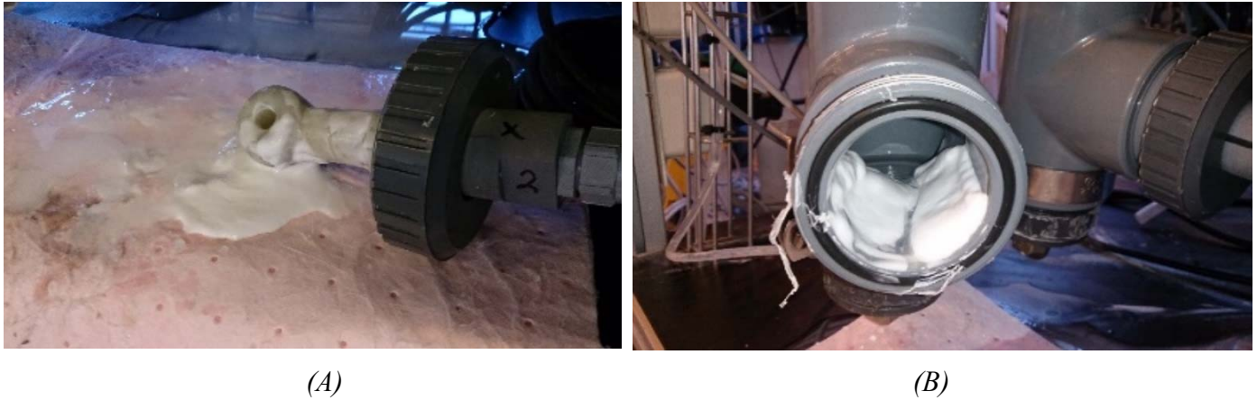
Figure 19. The precipitated salts in the system during the 2 mg/L dose of antiscalant. (A) Concentrate conductivity probe. (B) Its chamber.
