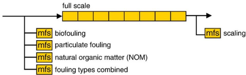
Figure 14. The position of MFS units to monitor different fouling types (Vrouwenvelder et al., 2011).
