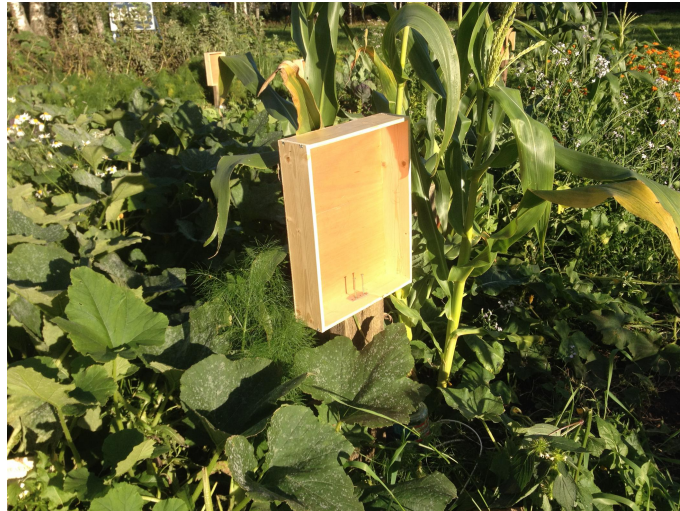
Figure 3.11 Speaker boxes were mounted on large wooden stakes bashed into the ground.
