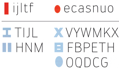
ILLUSTRATION 25: Different archetype shapes that are underlying often mistakable letters, as defined by Beier (2012, P. 73) . Geometric shapes such as rectangle, circle and triangle are common to letter groups, yet also introduce confusability. Image from Beier (2012) .
