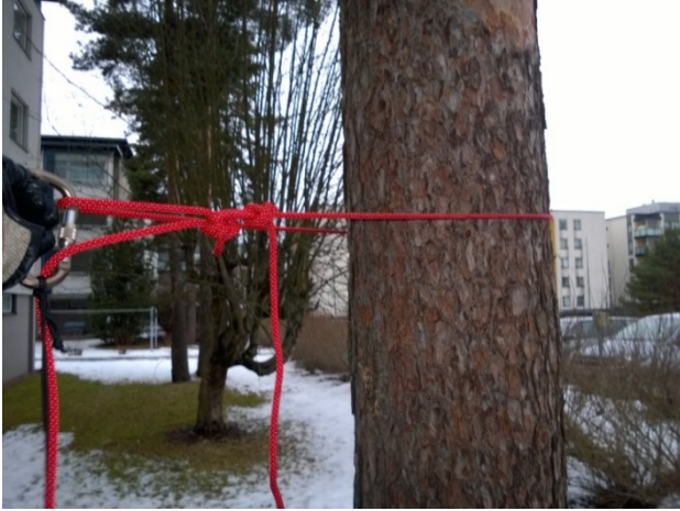
Figure 5-353: Test 2-B, Weight away from tree trunk, free fall device - setup
