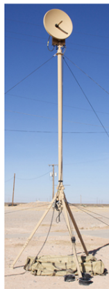
(a) Sectional mast with tripod base (Comrod Communication AS, 2016)
