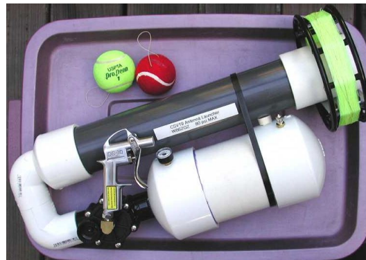
Figure 5.14: CSV19 pneumatic DIY antenna launcher (Alan Biocca Engineering, 2015)
