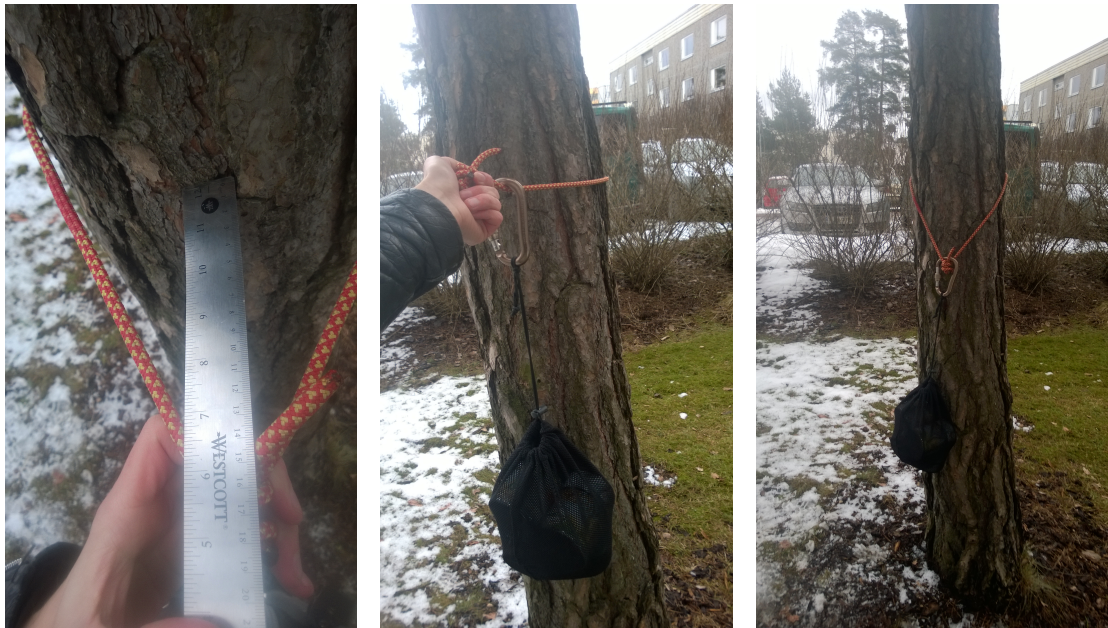
(a) Slack measurement of 15 cm (b) Payload pulled away from tree trunk (c) Payload secured by static loop
