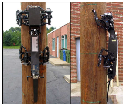
Fig. 1: Dorsal and lateral views of the RiSE Version 3 climbing robot. Four powerful legs, each with two actuators, grip a wooden telephone pole using claw-like appendages.
