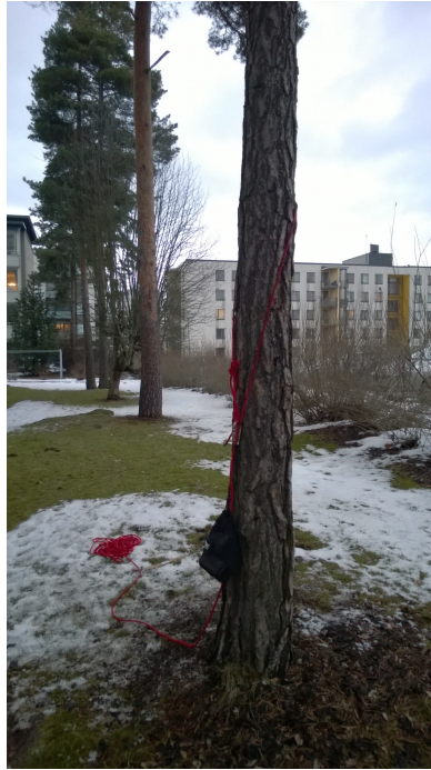
Figure 11.17: Static loop drop test - 73 cm diameter loop on 26 cm diameter tree trunk
