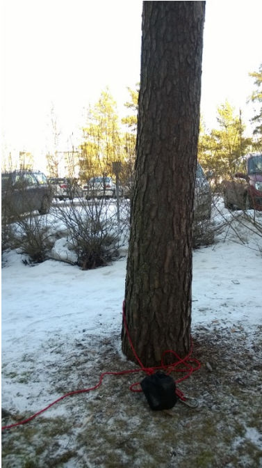
Figure 5-32: Test 1-B, Weight against tree trunk – “Pull Off” - not supported - result
