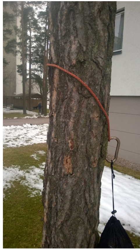
Figure 5-16: Static loop test b); result (approx. 18 cm drop)
