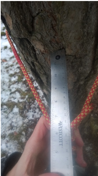
Figure 5-12: Static loop drop test slack measurement
