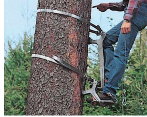
Figure 5.3: Swiss Tree Grippers (Forestry Suppliers, Inc., 2016)
