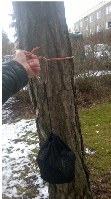
Figure 5-13: Static loop drop test a); weight pulled away from tree trunk
