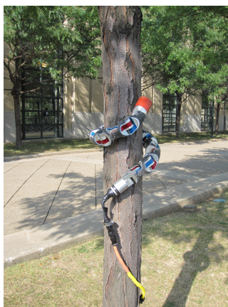
Figure 5.28: Snakebot climbing a tree (Biorobotics Lab, 2013)
