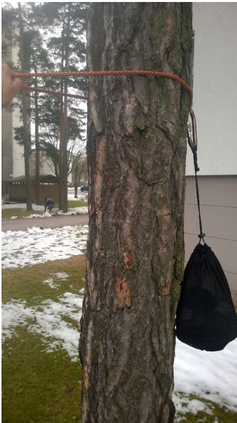
Figure 5-15: Static loop drop test b); weight against tree
