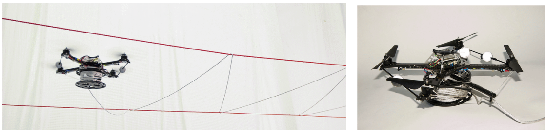
(a) Quadcopter constructing a rope structure
