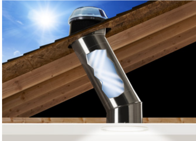
Figure 20 Structure of the light tunnel (Solatube 2015).
