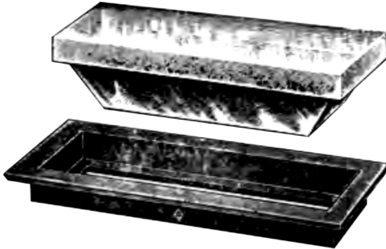
Figure 21 Deck prism's structure. Upper part is glass and lower brass or similar metal. Light enters from top and space below is illuminated (Davey 2016).
