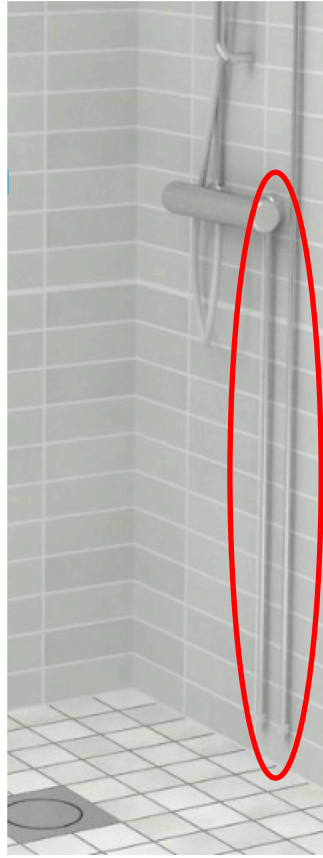
Figure 17 The additional plumbing required by the Ensavetec system. (Ensavetec 2016).
