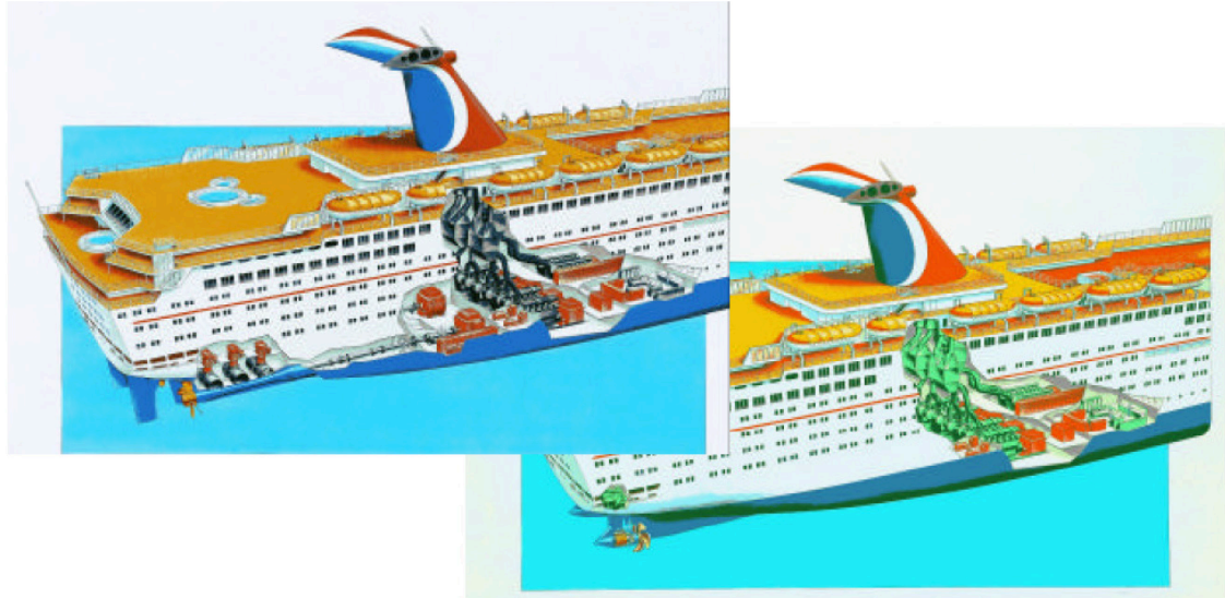
Figure 4 Cruise vessel with traditional shaft drive in the upper left picture and modern propulsion with electrical motor running the propeller in the lower picture (ABB 2003).
