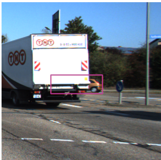
Figure 5.2: An example of a missing label in the KITTI dataset [6]. The bounding box prediction made by the network is counted as a false positive as the occluded car has not been labeled.
