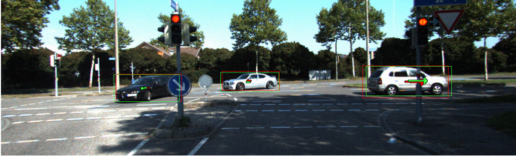
Figure 2.8: One validation frame from the KITTI tracking dataset [6]. Ground truth bounding boxes and velocity vectors are drawn in red and the detected objects and predicted velocity vectors are in green. The model has correctly predicted the velocity vectors for the cars based on their locations in the previous frames.
