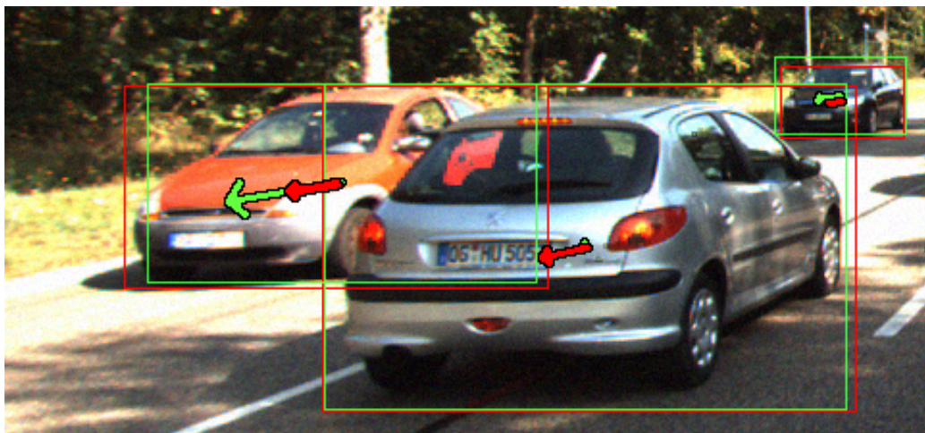
Figure 5.1: CNN model velocity prediction performance shown against a validation frame from the KITTI tracking dataset [6]. The predicted vectors are red and ground truth vectors are green. Interestingly, even though the CNN model has no temporal context across frames, it is able to make statistical guesses about car movement based on their orientation. The velocity of the car on the front is incorrectly marked by a vector pointing to the left even though in reality it is close to stationary. The model may have learned that cars driving on the next lane usually move towards the viewer.
