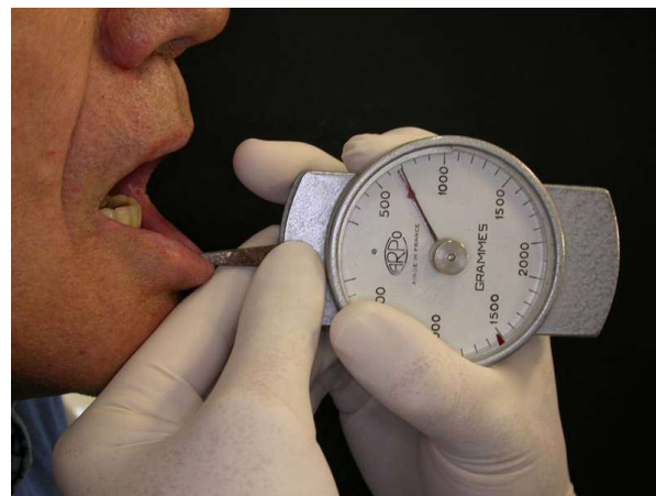
Fig. 1. The tip of a spring scale (Carpo, France) was placed at the margin of the dentures.
