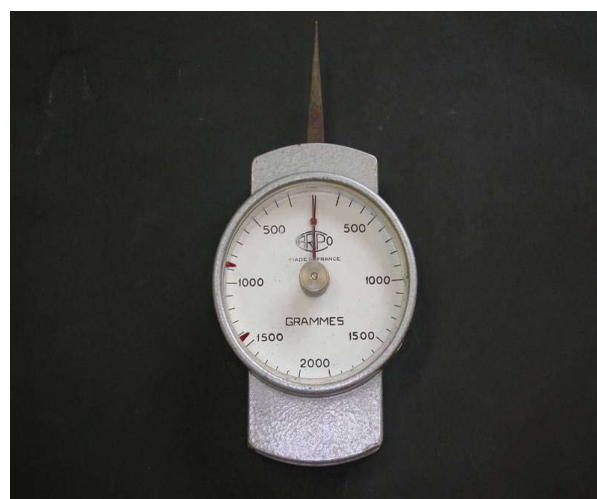
Fig. 2. The maximum retention force being registered by the spring scale.
