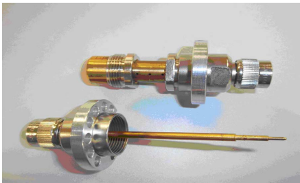
Fig. 1. Manufactured coaxial sample for multipactor test.
