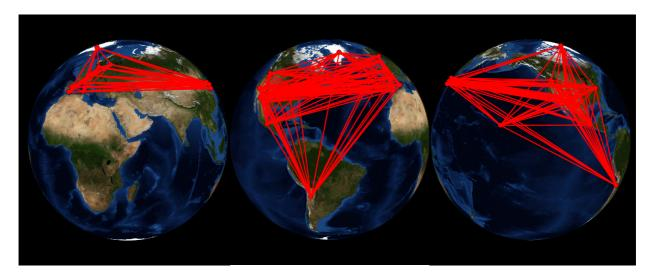
Figure 2: mmVLBI baselines at 86 GHz as viewed from M 87. The figure includes baselines with GMVA stations under development, the Sardinia Radio Telescope and the Large Millimeter Telescope in Mexico, and a future Greenland Telescope.
