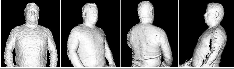
Figure 6.1 Surface reconstruction example with KinectFusion.
