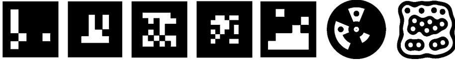
Figure 4.11 Some industry-standard visual makers. From left to right: Aruco, BinARyID, ARTag, ARToolkitPlus, Cantag, Intersense and ract-TIVsion.
