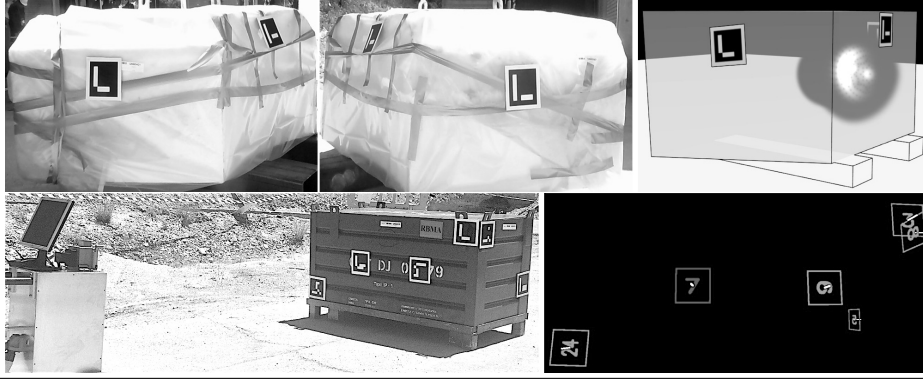
Figure 8.13 Irregular concrete piece and a waste container tracked with a marker map composed of visible fiducials.
