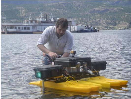
(a) Kingfisher M100 USV with mounted SONAR and omnidirectional sensors.
