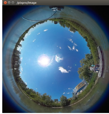
(b) A single measurement/image retrieved from the camera showing the cropping of image by the CMOS sensor
