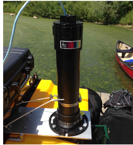
(b) Sensor mounted on the robot. The lower end of the sensor protrudes below the surface of the water. The internet connection to the onboard ROS infrastructure can be seen at the top of the sensor
