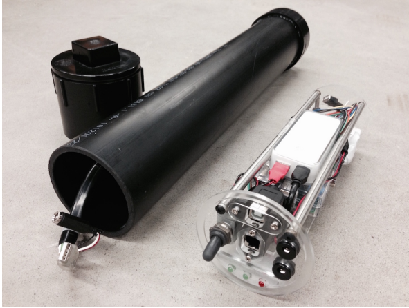
(a) Disassembled sensor showing: environmental housing, internal hardware structure, status LEDs and power/data ports.
