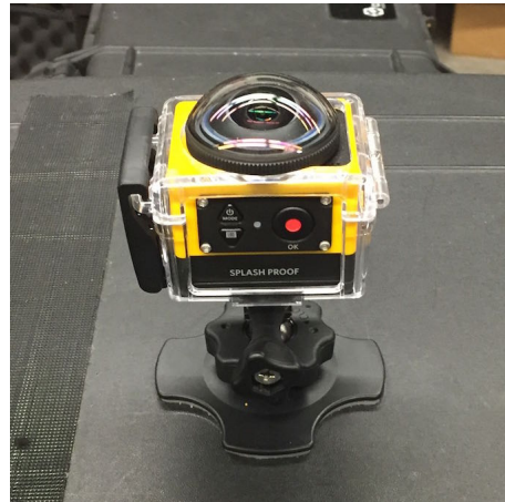
(b) Camera in a standard housing mounted to the robot using a ball and socket joint.
