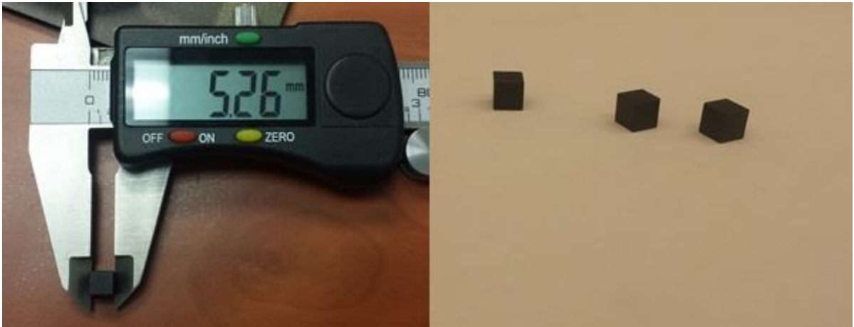
Figure 5-20 Delrin 150SA samples prepared for ASTM E 595 test
