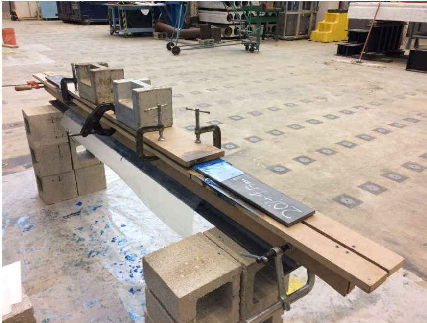
Rehabilitated beam after the application of clamps
