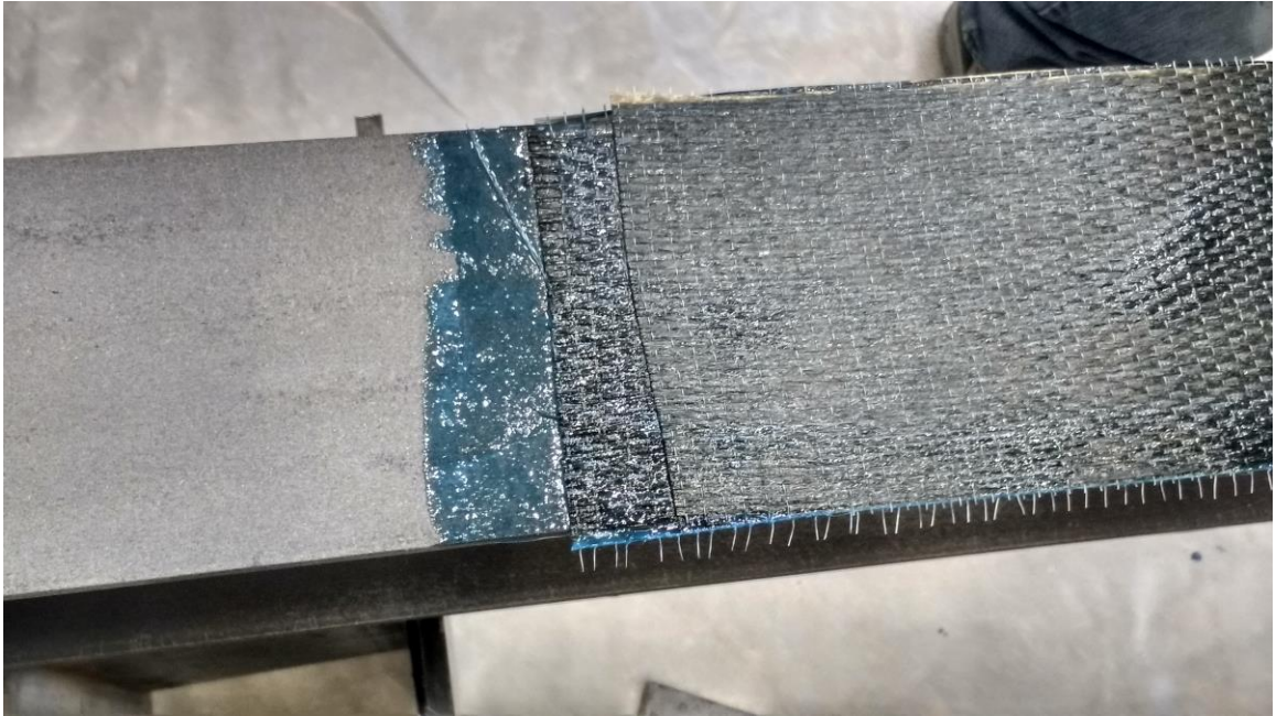
Tapering of longitudinal fabric endpoints between layers
