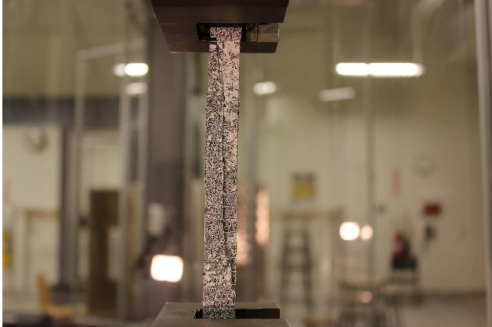
Figure 3.7: Basalt coupon after test
