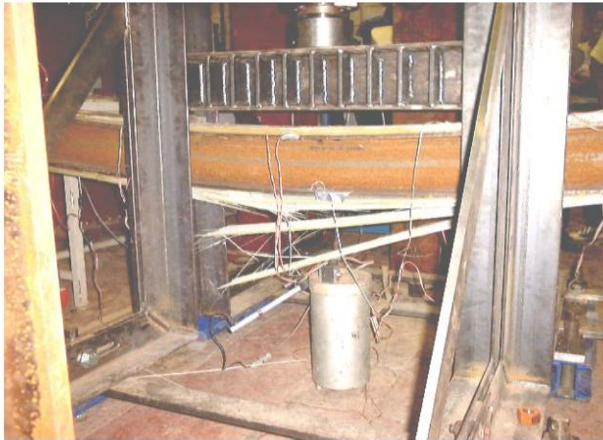
Figure 2.11: Failure of strengthened beam (El Damatty et al. 2003)
