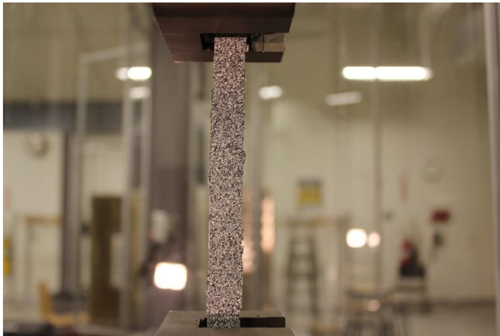
Figure 3.6: Basalt coupon before test
