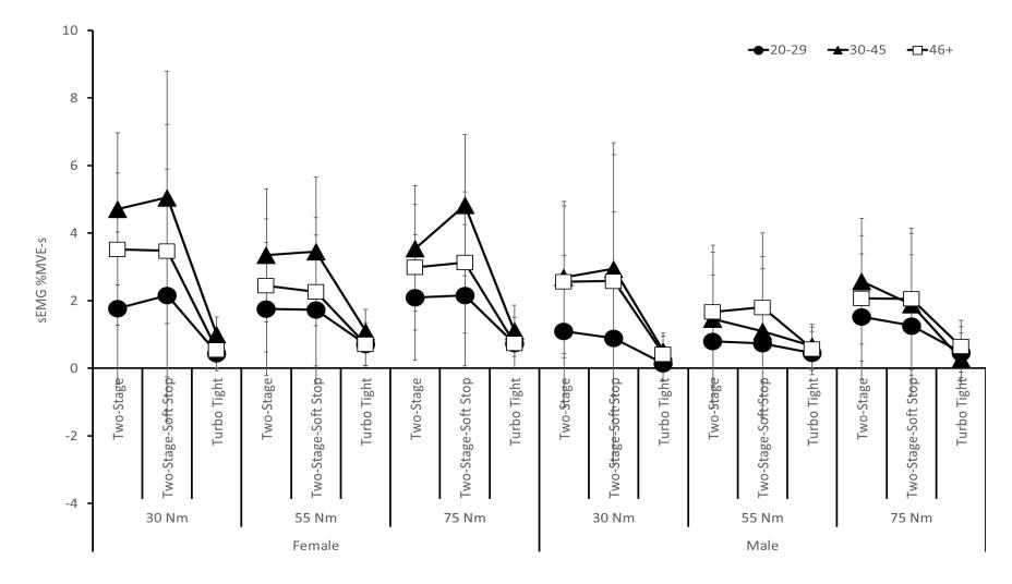
Figure 42: Right Upper Trapezius Impulse Magnitudes for Age, Gender, Target Torque and Fastening Strategy for Hard Joints. Significant interactions were seen for females aged 30-45 at 75 Nm between TSS and TT. Results reported on the sEMG %MVE-s means and standard error bars.
