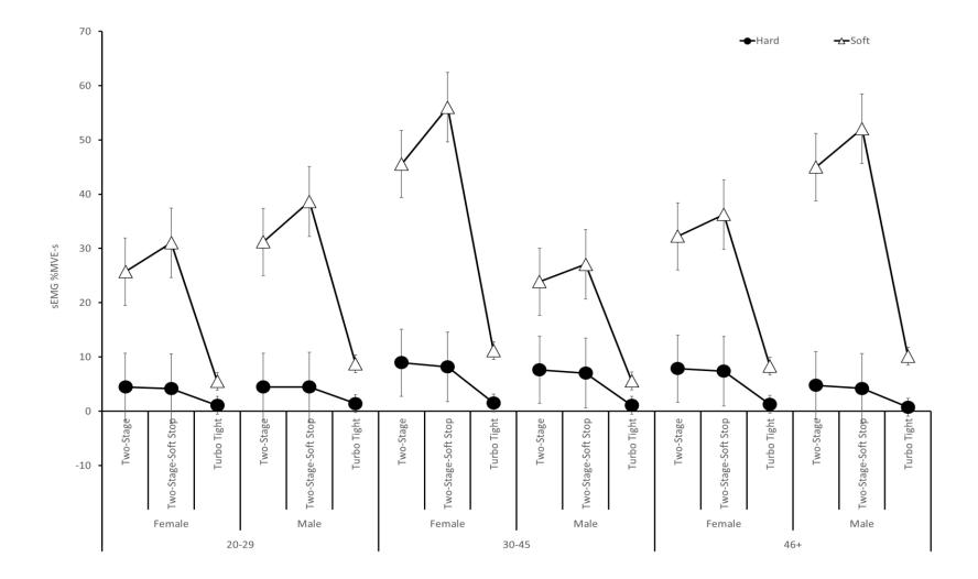
Figure 37: Right Flexor Carpi Ulnaris Impulse Magnitudes for Joint Hardness, Age, Gender and Fastening Strategy. Significant interactions between TS and TT and TSS and TT were seen by males age 30-45 and females aged 46+ fastening soft joints. Significances were also seen between TS and TT, TSS and TT and TSS and TS for females and males aged 20-29, females aged 30-45, and males aged 46+ fastening soft joints. Results reported on the sEMG %MVE-s means and standard error bars.
