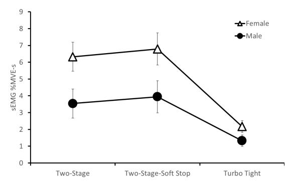
Figure 29: Right Anterior Deltoid Impulse Magnitudes for Gender and Fastening Strategy. Significant interactions were seen between tightening strategies TS and TT and TSS and TT for both males and females. Results reported on the sEMG %MVE-s means and standard error bars.
