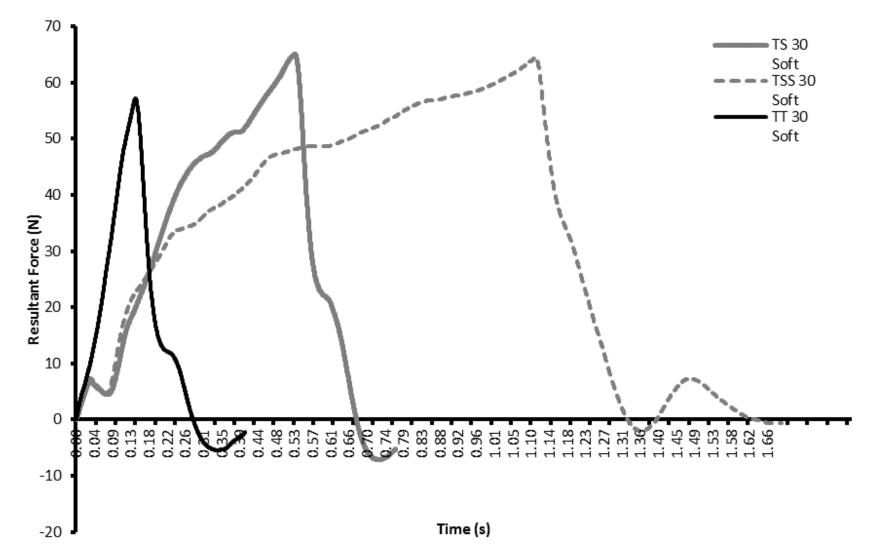
Figure 47: A visual representation of the three fastening strategies recorded by the RAPT handle for soft joints displaying the time periods and resultant forces for 30 Nm hard joints. This shows that the turbo tight fastening strategy takes place over a short period of time and results in a lower force occurring at the RAPT handle.
