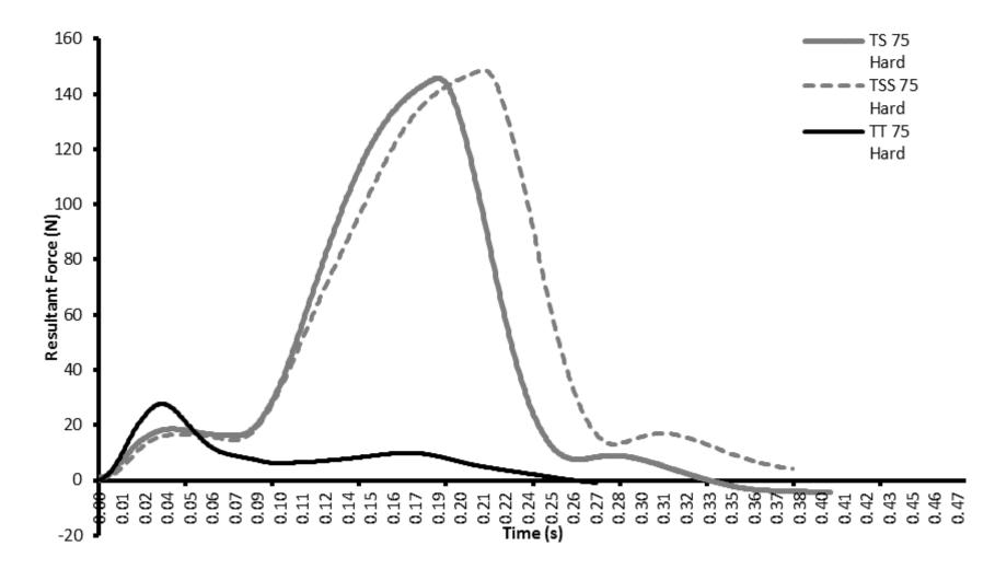
Figure 46: A visual representation of the three fastening strategies recorded by the RAPT handle for hard joints displaying the time periods and resultant forces for 75 Nm hard joints. This shows that the turbo tight fastening strategy takes place over a short period of time and results in a lower force occurring at the RAPT handle.
