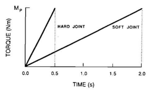
Figure 6: Torque buildup time for hard and soft-joints (Radwin et al., 1989) .
