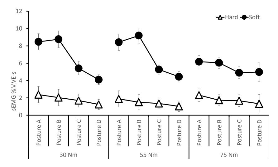
Figure 30: Right Anterior Deltoid Impulse Magnitudes for Joint Hardness, Fastening Location and Target Torque. Significant interactions were seen between postures A and C for hard joints at 30 Nm. Soft joints showed significant interactions between postures A and C, A and D, B and C, B and D and C for 30 Nm and 55 Nm joints. Soft joints at 75 Nm showed significances between postures A and D and B and D. Results reported on the sEMG %MVE-s means and standard error bars.
