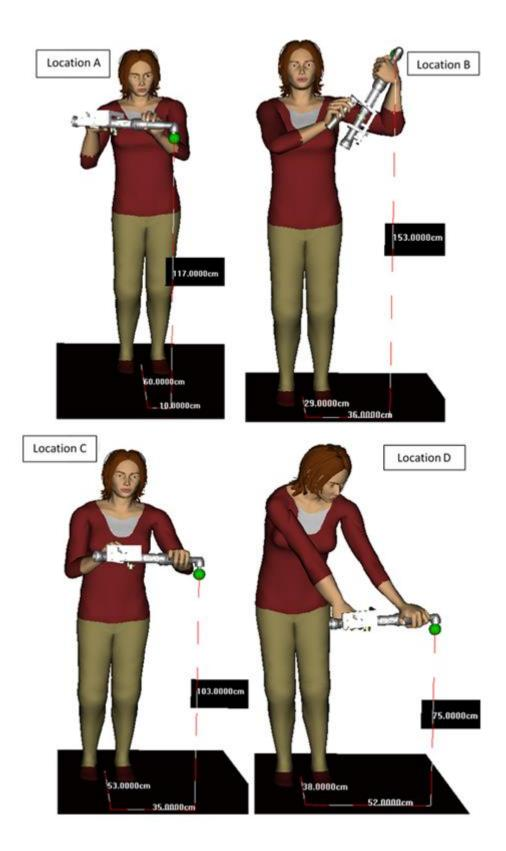
Figure 23: Portrayal of fastener location-orientation. This figure depicts the 4 locations and orientations as well as their geometrical locations with respect to the mid ankle position and the ground. Location ID: A, B, C, D.
