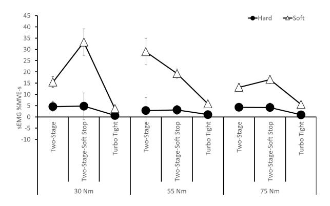
Figure 39: Right Pectoralis Major Impulse Magnitudes for Joint Hardness, Target Torque and Fastening Strategy. Hard joints at 30 Nm showed significances between TS and TT only. Significant interactions between TS and TT and TSS and TT for hard joints at 75 Nm and soft joints at 55 Nm. Significances were seen between TSS and TS, TS and TT and TSS and TT for soft joints at 30 Nm and 75 Nm. Results reported on the sEMG %MVE-s means and standard error bars.
