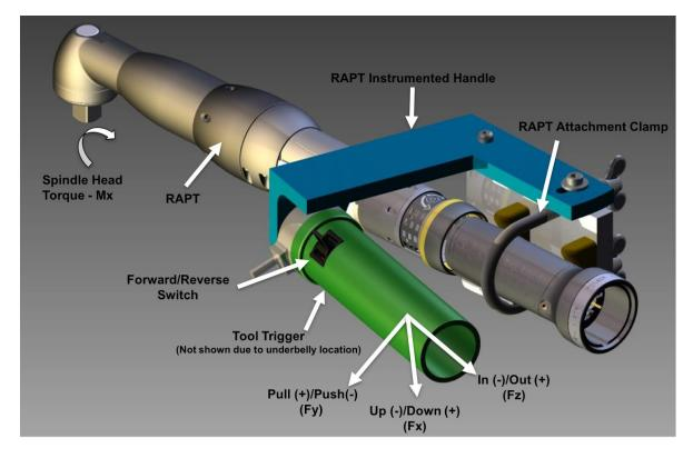
Figure 21:RAPT and Instrumented Handle Attached with Direction of Forces and components of the instrumented handle
