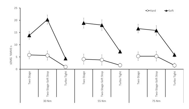
Figure 34: Right Extensor Carpi Ulnaris Impulse Magnitudes for Joint Hardness, Target Torque and Fastening Strategy. Significant interactions were seen between TS and TT and TSS and TT for hard joints at 30 Nm and 75 Nm and for soft joints at 55 Nm and 75 Nm. Soft joints at 30 Nm showed significant interactions between TS and TT, TSS and TT and TSS and TS. Results reported on the sEMG %MVE-s means and standard error bars.
