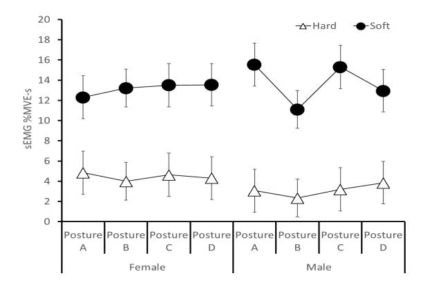
Figure 33: Right Extensor Carpi Ulnaris Impulse Magnitudes for Joint Hardness, Gender and Fastening Location. Females showed significant interactions between postures C and A for soft joints. Males showed significant interactions between postures A and B, A and C, D and B and D and C for soft joints. Results reported on sEMG %MVEs means and standard error.
