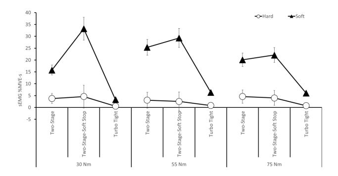
Figure 35: Right Flexor Carpi Radalis Impulse Magnitudes for Joint Hardness, Target Torque and Fastening Strategy. Soft joints at 55 Nm and 75 Nm showed significant interactions between TS and TT and TSS and TT. Soft joints at 30 Nm showed significant interactions between TSS and TT, TS and TT and TSS and TS. Results reported on the sEMG %MVE-s means and standard error bars.
