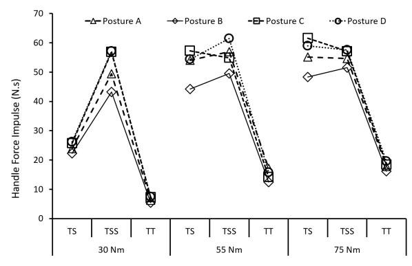
Figure 27: Handle forces magnitudes for posture, target torque and fastening strategy for soft joints. Significances seen between TS and TT and TSS and TT for all postures and target torques. Significances seen between TS and TSS for posture A at 30 Nm, posture B for all target torques, posture C for 30 and 75 Nm and posture D for 30 and 55 Nm.
