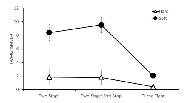
Figure 40: Right Triceps Brachii Impulse Magnitudes for Joint Hardness and Fastening Strategy. Significant interactions were seen for soft joints between TS and TT and TSS and TT. Results reported on the sEMG %MVE-s means and standard error bars.
