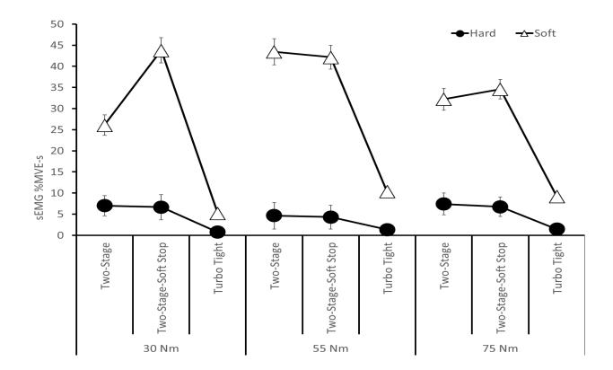
Figure 38: Right Flexor Carpi Ulnaris Impulse Magnitudes for Joint Hardness, Target Torque and Fastening Strategy. Significant interactions between TS and TT and TSS and TT were seen between hard joints at 30 Nm and 75 Nm and soft joints at 55 Nm. Significances were seen between TSS and TS, TS and TT and TSS and TT for soft joints at 30 Nm and 75 Nm. Results reported on the sEMG %MVE-s means and standard error bars.
