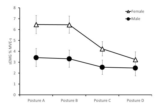
Figure 28: Right Anterior Deltoid Impulse Magnitudes for Gender and Fastening Location. Significant increases were seen between males for postures A and A and B and D and female for postures A and C, A and D and B and C. Results reported on the sEMG %MVE-s means and standard error bars.
