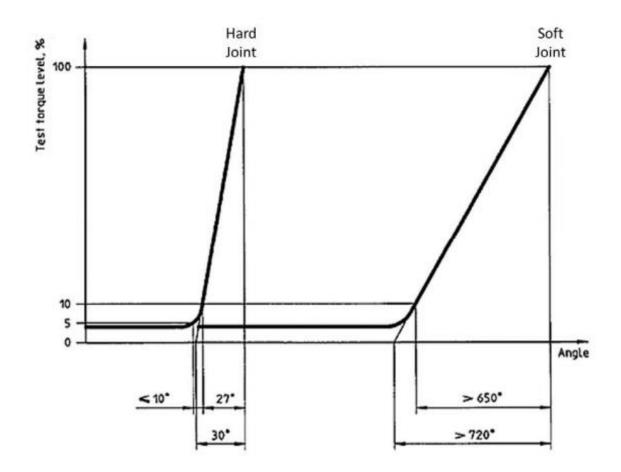
Figure 5: Spindle head angle vs. torque level in hard and soft-joints (International Standards Organization, 1994).
