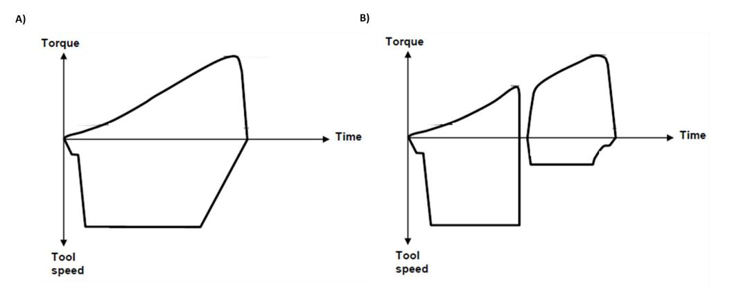
Figure 2: Tightening profiles: A) One stage with one constant velocity B) Two stage with high speed first step, a break and a lower speed second step (Atlas Copco, 2013b).
