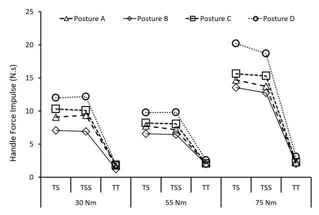
Figure 26: Handle forces magnitudes for posture, target torque and fastening strategy for hard joints. Significances seen between TS and TT and TSS and TT for all postures and target torques.
