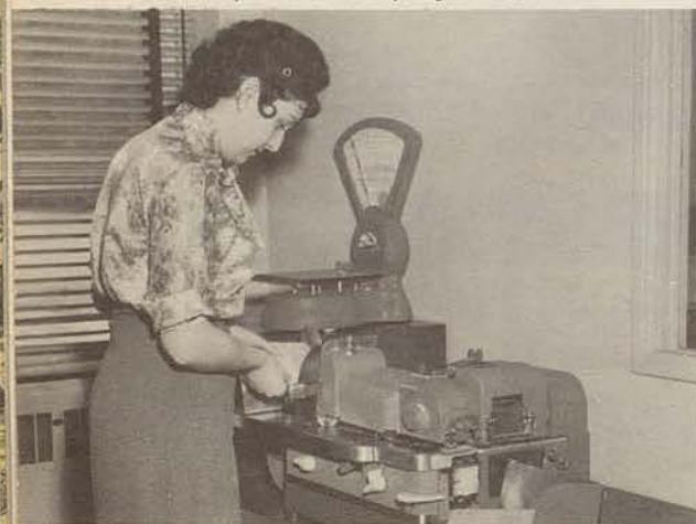
One person operating this folding machine performs a task in 10 days, which, prior to mechanization, took 7 persons 25 days to complete.
