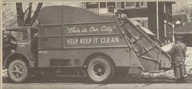
A major improvement in refuse collection has been achieved by the replacement of the open truck by the more sanitary enclosed packer-type vehicle.
