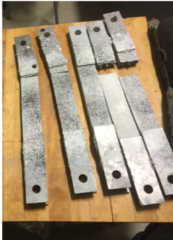
Figure 4.2 Failure of G-FRCM coupons
