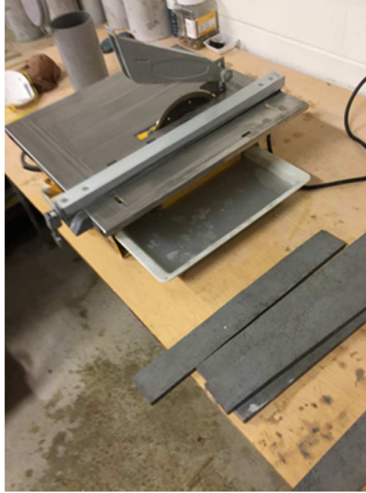
Figure 3.2 Cutting FRCM panel using wet-diamond saw
