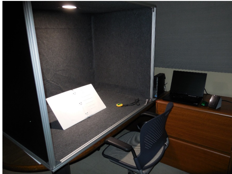
Figure 2. Actual light test box device at the university setting
