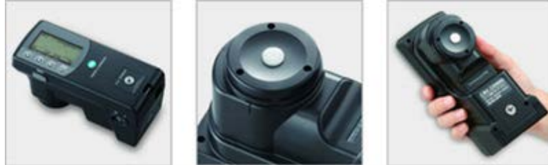
Figure 9. The CL-500A Illuminance Spectrophotometer
