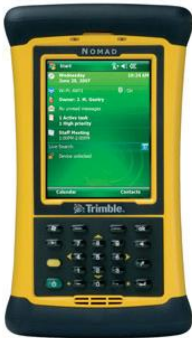
Figure 17 – (left to right) (a) A display of the Trimble Nomad GPS Unit; (b) display of GPS unit used in acquiring geographic coordinates for a gravity station in the field.
