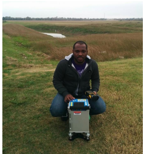
Figure 15 - (left to right) (a) The top view of CG-5 Scintrex Autograv (b) displays the field set-up of the CG-5 gravity meter before a gravity measurement is taken. The gravity meter is mounted on a tripod which comes with a rotating foot screw used for adjusting for tilt. When adjusted within a range of \pm 10 arcsec, a cross hair and an icon is displayed as shown in figure 15a.
