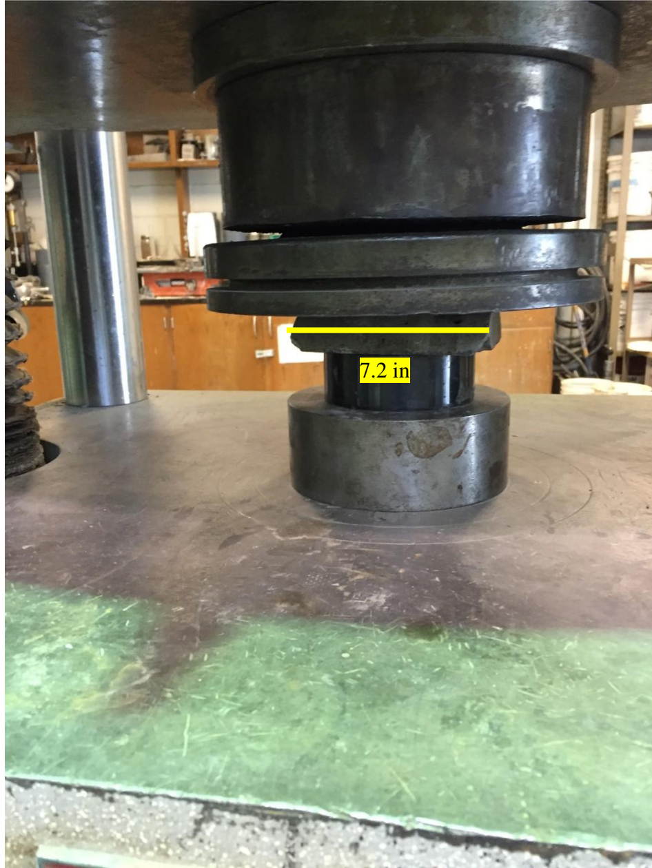
Figure 14—Equipment used for testing the compressive strength and tensile strength at University of Houston’s Civil Engineering Laboratory. The same equipment is used to test the UCS and Tensile strength and the samples are rested on the instrument depending upon the test and the load is applied.
