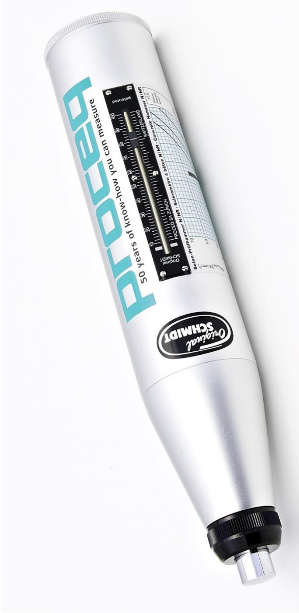
Figure 10–N type Schmidt Hammer, where A is the needle which is placed at the surface of the rock and B is scale of the hammer which is used to measure the strength in MPa (PCTE, 2016)
