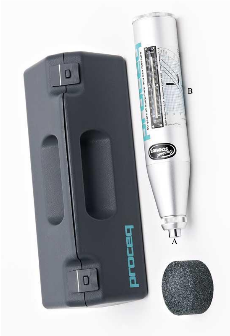
Figure 9 –L type Schmidt Hammer, where A is the needle which is placed at the surface of the rock and B is the scale of the hammer which is used to measure the strength in MPa (Proceq, 2016).
