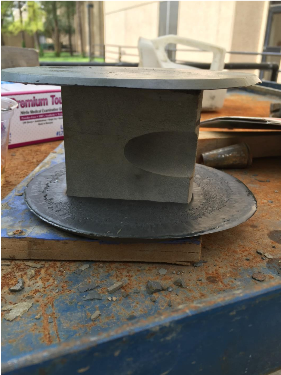
Figure 17–Top and bottom of the samples are flattened by adding Sulfur which is melted at 300° F. Cores are made flat so that they are stable when subjected to stress.
