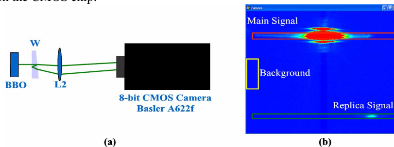
Fig. 3. (a). Using a 1^\circ uncoated wedge a signal replica with an intensity decrease of a factor of 0.0018 is created. (b) CMOS camera image (of the single-shot autocorrelator) showing the three areas used for the signal retrieval.
