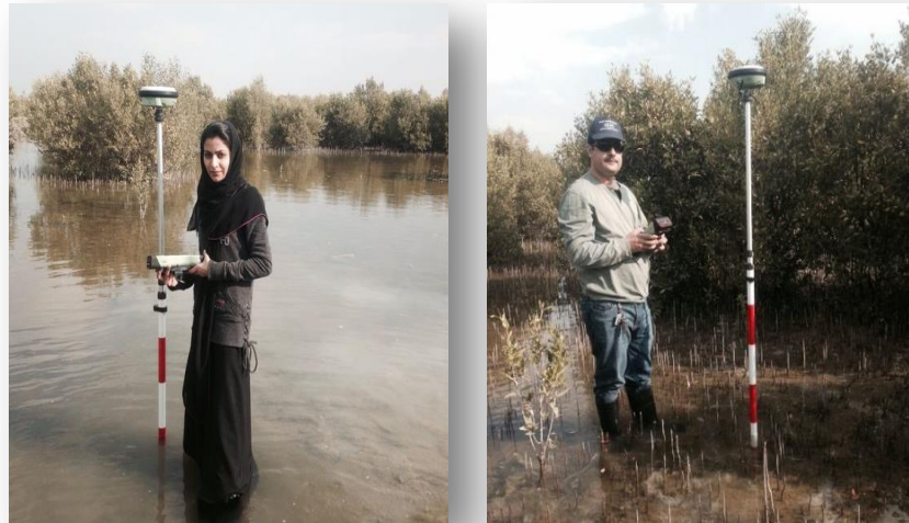
Figure 4. Determining the locations of ground plots using Leica Viva GS14 GNSS RTK receiver in January, 2014.
