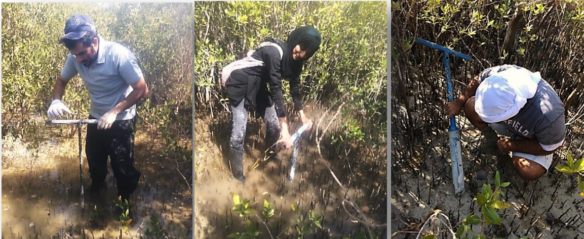
Figure 16: Collecting soil samples using augers in February 2014.
