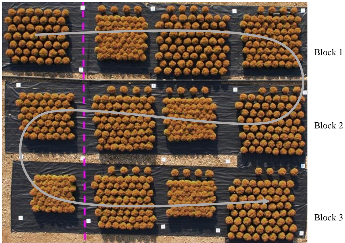
Fig. 2.2. Aerial image of the experimental layout. The gray line represents the flight path or run for the UAV.
